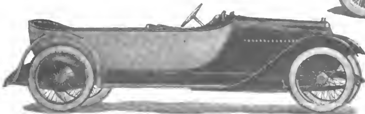
Aquatic touring body by Holbrook. The general lines are like those of a boat. It is mounted on a DeDion-Bouton chassis
